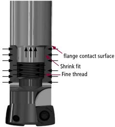
Our Pokolm DuoPlug® system offers optimum rigidity and extremely high precision and concentricity. As a supplement to conventional thread connections, the retention and supporting forces between cutting tool and adapter act along the entire surface of the shrink fit and a large part of the shrink thread.For more information, please see the assembling and dismantling instructions for our DuoPlug® system in the "Operation Data" chapter.
